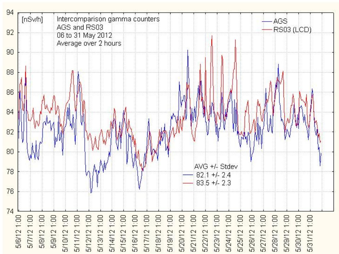
Fig.2 Time series of both dose-rate measurement series (312 data points)
