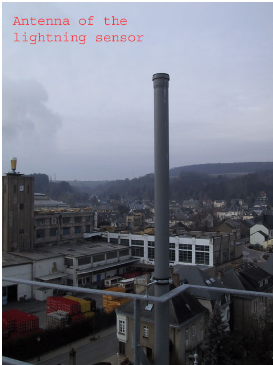
Fig.1. Antenna system of the Boltek Storm Tracker. The antenna module is mounted inside a PVC tube for rain and environmental protection.
