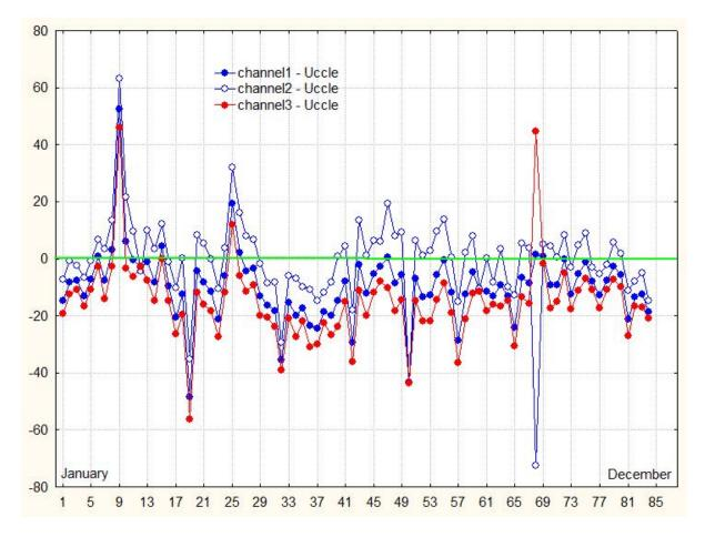
fig. 5 Differences (channel x - Uccle) during 2012. Time interval between successive points is variable!
