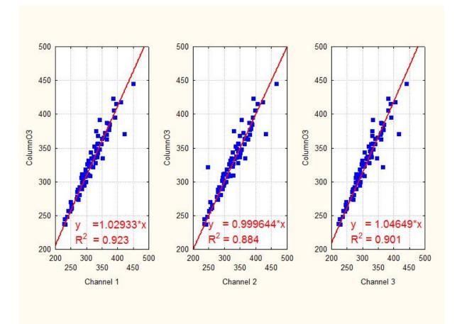
fig. 2 Uccle DS versus the three Microtops channels (N = 84 data points)
