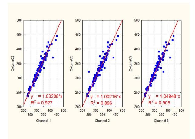
fig. 1 Uccle DS & ZS versus the 3 Microtops channels (N = 98 data points)
