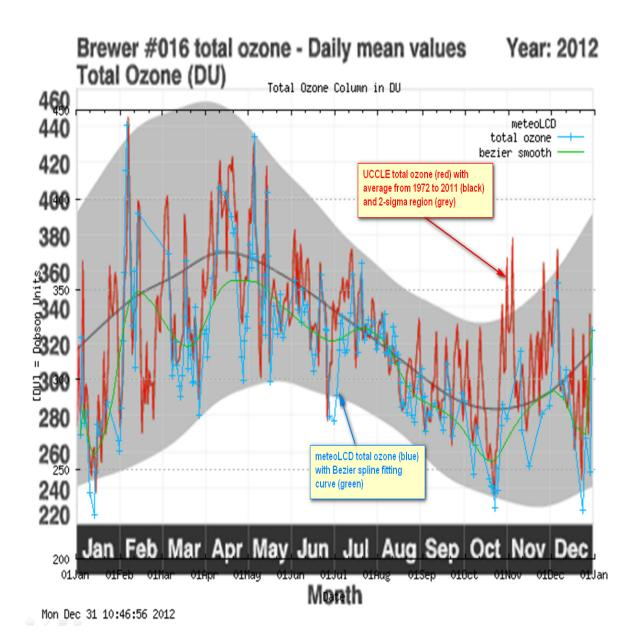
fig. 7. Overplot of the website plots of the Uccle and Diekirch TOC measurements at the end of the year 2012. The grey area corresponds to the 2-sigma region around the averagesat Uccle from 1971 on.
