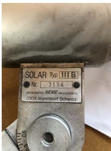
Fig.1 Serial plate of a 111B type sensor (with MIL connector)
