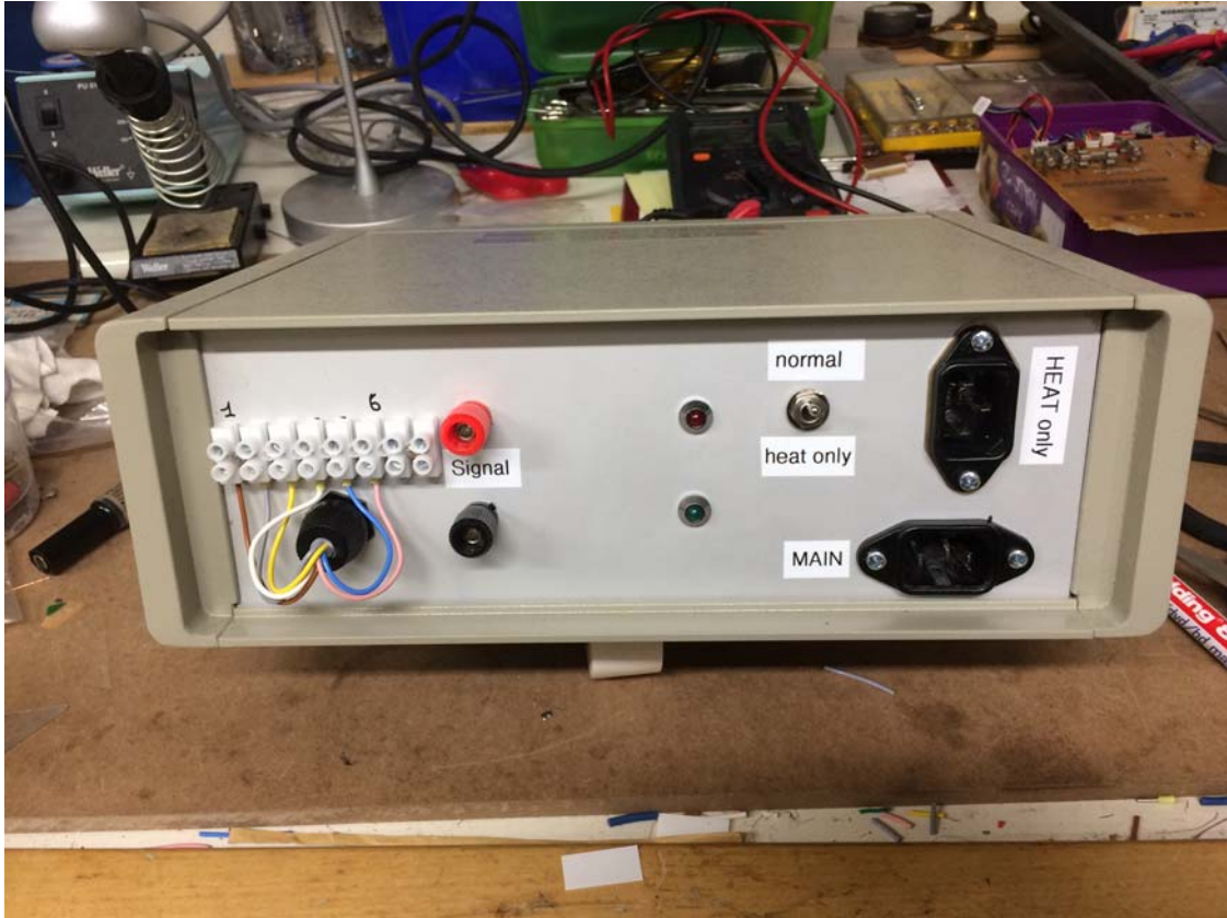
Fig.8. The home-made power supply for the Haenni Solar 111
