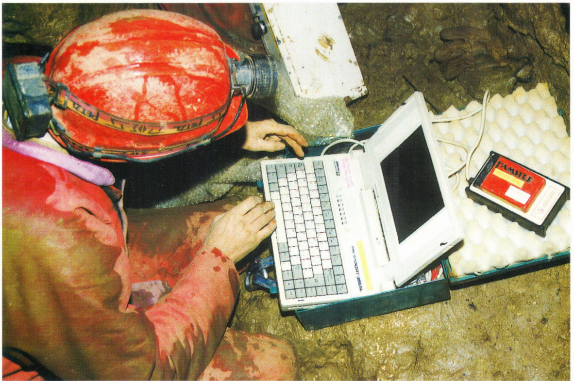
K Downloading th temperature data from the stand-alone Hamster logger.
