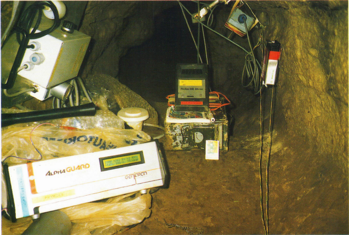
L Miscellaneous instrments at Station 4. From left to right: Dew Point Sensor, Alphaguard, Dosimeter & WL-Meter (Rn), Barometer and Temp. Logger
